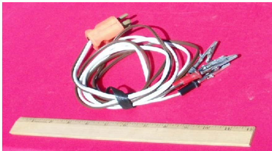
The Pad Cables with Alligator clips 2 sets are required for 4 pads
