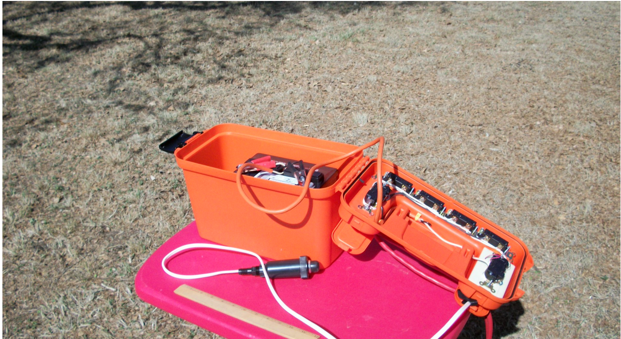
The Launch Controller connected to an internal lead acid battery
